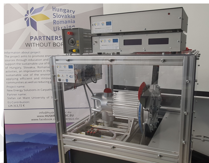
Three-phase wind turbine/Wind simulator- EOLYS 500 Turbină eoliană trifazată/Simulator eolian EOLYS-500
